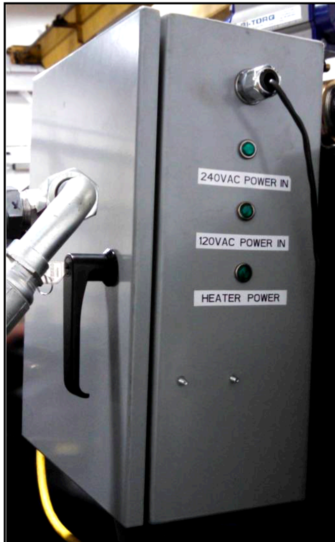
Figure 9.4 Emulsion Tank Heating System LED Locations
